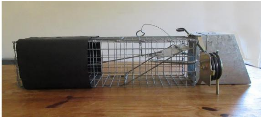
Photo 4. The Kania 2000 attached to a standard squirrel trap, two springs hold the two traps close together to avoid escapes.
