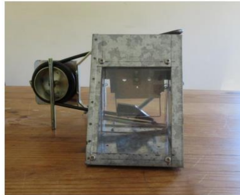
Photo 5. The Kania 2000 with the back cut out of the housing and Perspex window inserted to encourage the squirrel to run toward the light.
